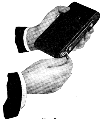
FIG. 7 Turning a new section of film into position.
